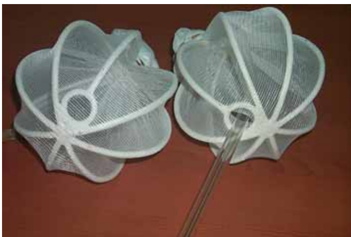
Figure 3. Bioassay procedure using wire frame for netting material (courtesy of Dr Mark Rowland, London School of Hygiene and Tropical Medicine, UK).
